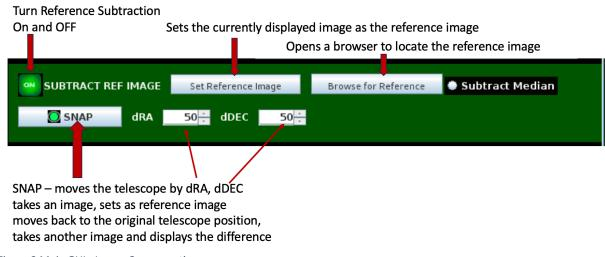
Figure 9 Main GUI - Image Compensation
